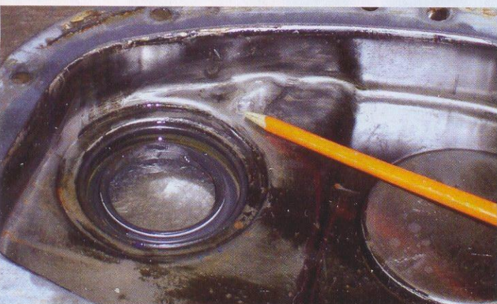
9. The other modification is to the timing cover, if it's an A-plus variant with the service tool bracket on the outside. There's a small protuberance inside the cover caused by the pressing in this area, and if not dealt with it rubs on the wider duplex chain. Simply tap it out with a ball pein hammer or with a drift.
