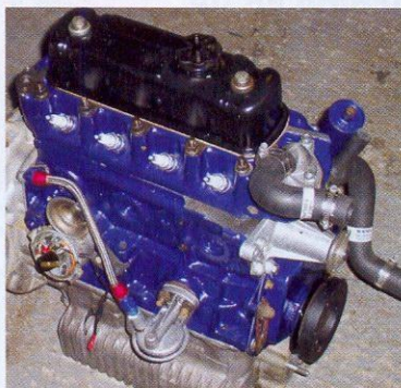
19. The finished assembled engine ready for installation. Note the flow-efficient block to filter head transfer pipe. I really don't like the standard set-up — it's very restrictive.
