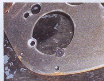
8. They need replacing with counter-sunk type screws/bolts. Ideally use either a proper countersink bit with a 45-degree taper to countersink the area around the retaining bolt holes so that the countersunk-type screws/bolts fit flush with the front plate.
